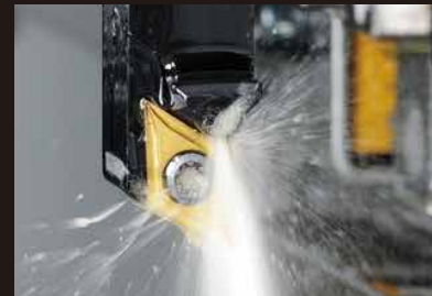
Internal coolant system
