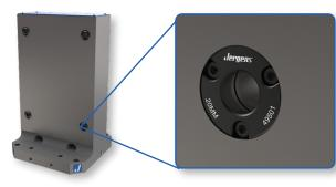
Ball-Lock® is Jergens most popular quick change system. Adding receiver bushings to the face of a column provides a method of quickly and accurately locating fixtures onto column surfaces. Reducing set-up time, fixtures can often be exchanged in less than a minute and positioned with repeatability of +/-.0005" (.013mm)
