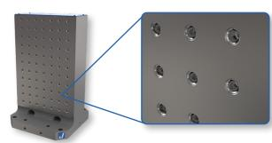
Adding precision bushings to each hole allows for accurate positioning with dowel pins or shoulder screws. Jergens QLS grid pattern provides fast and accurate mounting for a wide range of standard top tooling from our popular modular systems like Quick-Loc™
